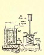
Fig. 248.—The circulating-oil-type transformer.
